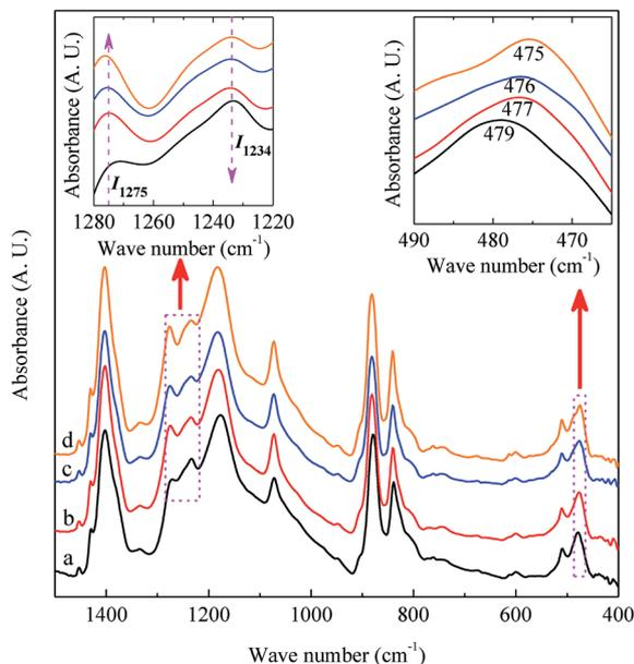
Fig. 6 FTIR spectra of electrospun membranes using 12 wt% of PVDF mixed with different  $V_{\text{NMP}}/V_{\text{acetone}}$  at 3/7, 4/6, 5/5, and 6/4 as labeled with 'a', 'b', 'c' and 'd', respectively. Insets are the magnification of frequency regions in 1220–1280  $\text{cm}^{-1}$  (left) and 465–490  $\text{cm}^{-1}$  (right). The arrows in the left inset indicate the direction of an increase in absorption.
