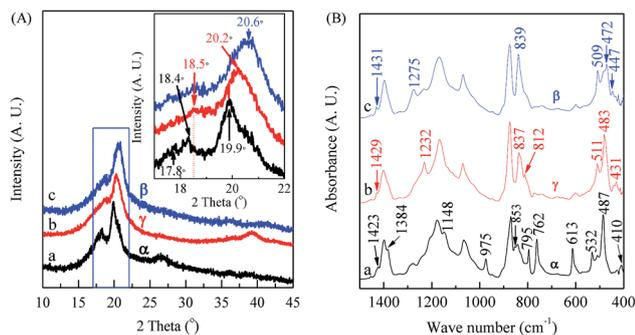
Fig. 4 XRD patterns (A) and FTIR spectra (B) of membranes cast from 8 wt% PVDF solution with  $V_{\text{NMP}}/V_{\text{acetone}}$  at 9/1: curve 'a' (black) for the sample dried at 150 °C; curve 'b' (red) for the sample dried at 40 °C; curve 'c' (blue) for the sample dried at 40 °C and drawn at 80 °C with a draw ratio of ca. 4.
