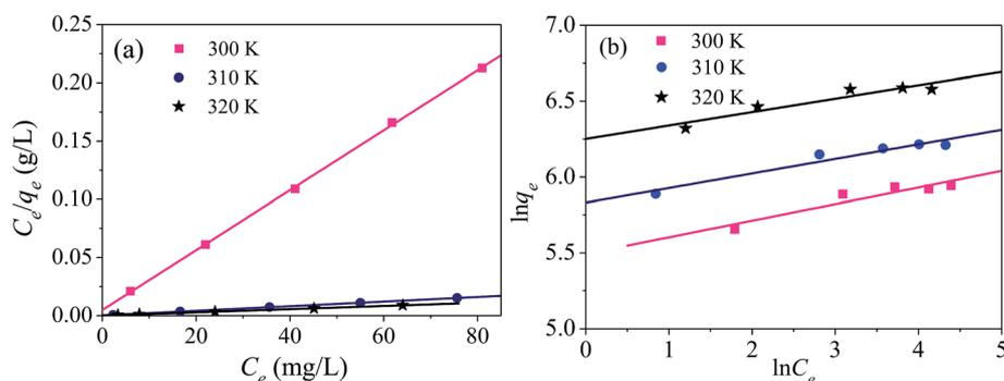
Fig. 14 Adsorption isotherms for the adsorption of mercury(II) onto magnetic PPy-GO: Langmuir (a) and Freundlich (b) models. Conditions: pH = 7 ± 0.1, RSL = 0.05 g L<sup>-1</sup>, C<sub>0</sub> = 20–100 mg L<sup>-1</sup>.
