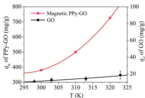
Fig. 13 Adsorption isotherms of mercury(II) onto the magnetic PPy-GO nanocomposite. Conditions: pH = 7 ± 0.1, RSL = 0.05 g L<sup>-1</sup> and C<sub>0</sub> = 100 mg L<sup>-1</sup> for the magnetic PPy-GO; pH = 6, RSL = 0.5 g L<sup>-1</sup> and C<sub>0</sub> = 100 mg L<sup>-1</sup> for the GO.<sup>32</sup>
