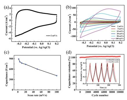
Fig. 5 The results of TCTL-II (a) at a scan rate of 2 mV s<sup>-1</sup>, and (b) at different scan rates. (c) Volumetric capacitance as a function of scan rate. (d) The cycling performance of the TCTL-II electrode at a current density of 5 A g<sup>-1</sup>. The black and red GCD voltage profiles of the TCTL-II electrode shown in the inset represent the first five cycles and the last five cycles, respectively.
