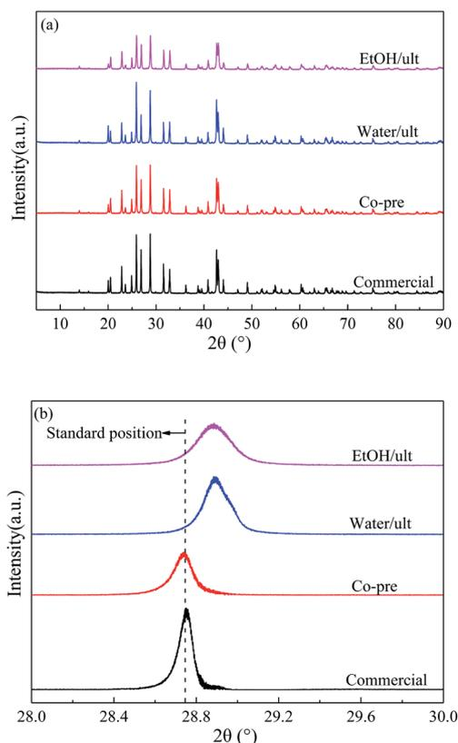
Fig. 1 (a) XRD patterns and (b) enlarged (121) diffraction peaks of BaSO<sub>4</sub> catalysts prepared with different methods.
