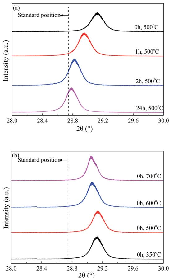
Fig. 2 Enlarged XRD (121) diffraction peaks of BaSO<sub>4</sub> catalysts (a) aged with varied time length and (b) calcined at different temperature.
