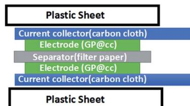
Scheme 1 Structure of the flexible supercapacitor device.
