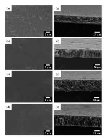
Fig. 4 Top view (a-d) and cross-section (e-h) SEM images of the PI membrane (a and e) and GO/PI MMMs with 0.5 wt% (b and f); 1 wt% (c and g), 2 wt% (d and h) GO loading
