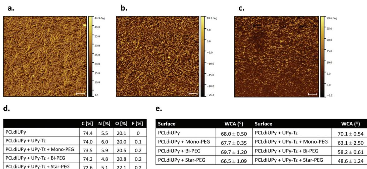
**Fig. 2** Surface characterization of the different material films with AFM, XPS and water contact angle. AFM phase micrographs of PCLdiUPy (a), PCLdiUPy with 10 mol% UPy-Tz (b) and after star-PEG-BCN functionalization (c), (d) XPS compositional table of the different surfaces and (e) water contact angles of the respective surfaces. Five measurements were performed per surface and standard deviations are plotted.
