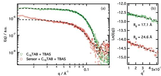
Fig. 4 (a) Small-angle X-ray scattering data and best fits (black-dashed lines) to the model described in the text of CTAB/TBAS before (green) and after (red) the incorporation of the **Az-1-Bpin** indicator (b) Guinier plot.
