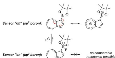
Scheme 1 Rehybridization of boron upon analyte binding.
