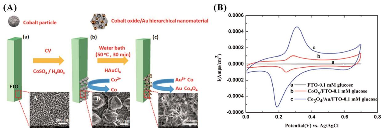
Fig. 5 (A) Shows the fabrication of  $\text{Co}_3\text{O}_4/\text{Au}$  hierarchically nanostructured electrode, and (B) presents cyclic voltammograms of the bare FTO,  $\text{CoO}_x/\text{FTO}$ , and  $\text{Au}/\text{Co}_3\text{O}_4/\text{FTO}$  in 0.1 M NaOH solution with the presence of 0.1 mM glucose. Adapted with permission from ref. 112. Copyright © 2016 American Chemical Society.
