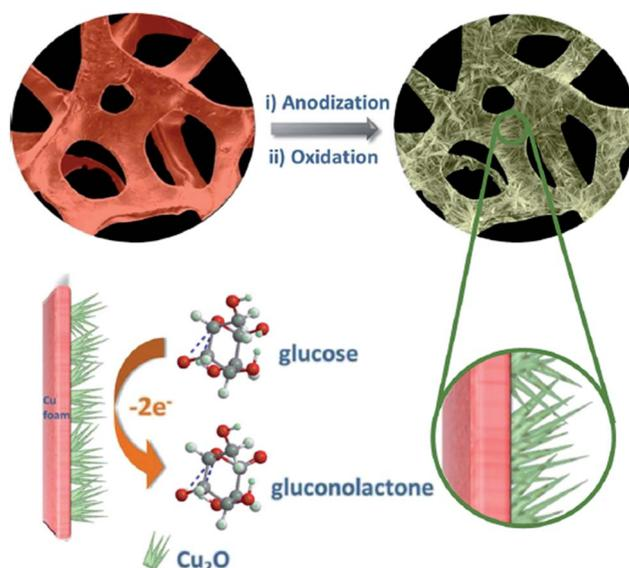
Fig. 4 Schematic illustration of the fabrication of the 3D Cu foam-supported mesoporous Cu<sub>2</sub>O nanothorn array electrode and its function in the electrocatalytic oxidation of glucose in alkaline media. Adapted with permission from ref. 19. Copyright © 2015 American Chemical Society.
