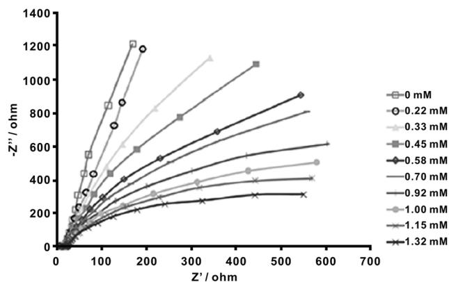
Fig. 3 Nyquist plots of Ni(OH)<sub>2</sub> thin film on Au electrode in 0.1 M KOH solution for glucose in the 0–1.32 mM concentration scope. Adapted with permission from ref. 69. Copyright © 2016 Elsevier B.V.
