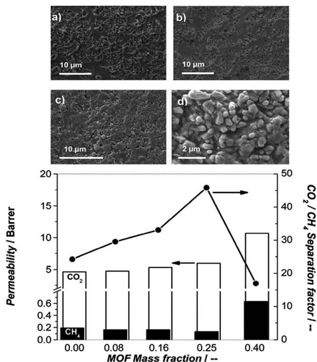
Fig. 13 SEM micrographs of the cross section of mixed matrix membrane containing 8 (a), 16 (b), 25 (c) and 40 (d) wt% NH<sub>2</sub>-MIL-53(Al) crystals. Reprinted from ref. 92 with permission from Royal Society of Chemistry.
