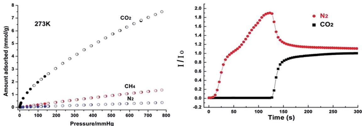
Fig. 7 (Left) Adsorption isotherms for CO<sub>2</sub>, N<sub>2</sub> and CH<sub>4</sub> at 273 K. (Right) Breakthrough experiment of an equimolar CO<sub>2</sub>/N<sub>2</sub> mixture at 0.1 MPa and 273 K. Reprinted from ref. 41 with permission from Royal Society of Chemistry.
