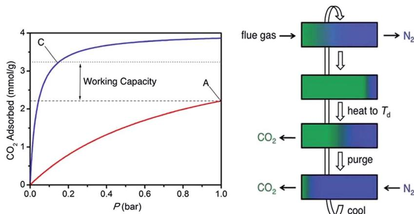
Fig. 10 (Left)  $\text{CO}_2$  adsorption isotherms at  $40^\circ\text{C}$  and  $150^\circ\text{C}$ . Reprinted from ref. 59. Copyright 2012 American Chemical Society. (Right) Schematic representations of temperature swing adsorption. Reprinted from ref. 73 with permission from Royal Society of Chemistry.
