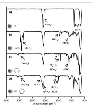
Fig. 2 FT-IR spectra of (A) hydride terminated SiNCs: SiNCs functionawith (B) n-hexyllithium; (C) phenyllithium; (D) phenylacetylide.
