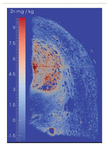
Fig. 2  $\,$  Zn distribution of a prostate cancer section analysed by LA-ICP-QQQ and an  $\,$  O $_2$  tune.
