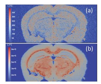
Fig. 3 (a)  $^{80}$ Se  $\rightarrow$   $^{80}$ Se $^{16}$ O image and (b)  $^{31}$ P  $\rightarrow$   $^{31}$ P $^{16}$ O image of a mouse brain obtained with LA-ICP-QQQ and an O2/H2 tune.
