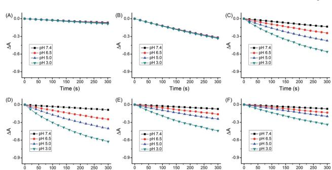
Fig. 4 Rate of decay of ABDA sensitized by (A) control, (B)  $[Ru(bpy)_3]Cl_2$ , (C) **1**, (D) **2**, (E) **3** and (F) **4** in aerated disodium hydrogen phosphate/citric acid buffer solutions as shown by the decrease in the absorption maxima of ABDA (377, 378, 380 and 380 nm for pH 3.0, 5.0, 6.5 and 7.4, respectively).
