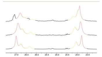
Fig. 7 Illustrative  $^{13}$ C NMR spectra of 7a (top), 7b (middle) and 7c (bottom) in 9:1 methanol: chloroform, with peaks arising from the 100%, 50% and 25% labels indicated by colours used in Fig. 6.
