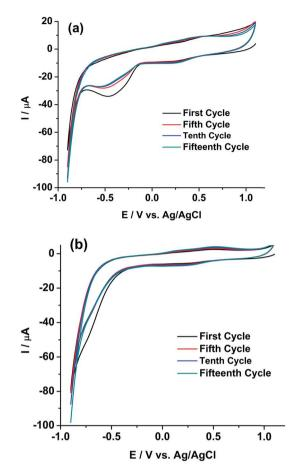
Fig. 8 Cyclic voltammograms of 5 mM U(vi) in 1 M  $H_2SO_4$  on (a) rGO/GC and (b) GC electrodes at a scan rate of 50 mV s<sup>-1</sup> for (i) first, (ii) fifth, (iii) tenth and (iv) fifteenth cycle.
