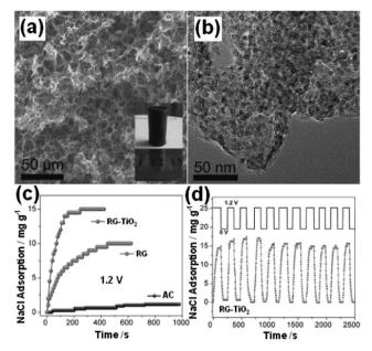
Fig. 20 (a) SEM and (b) TEM images of the RG-TiO $_2$  composite; (c) the desalination efficiency of AC, RG and RG-TiO $_2$  in 500 mg L $^{-1}$  NaCl solution at different times; (d) electrosorption and regeneration cycles of RG-TiO $_2$  in 500 mg L $^{-1}$  NaCl solution. (Reproduced with permission from ref. 50.)
