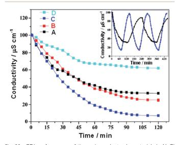
Fig. 22 CDI performance of the various electrode materials in NaCl solution at 1.2 V. (A) RG, (B)  $MnO_2$  NPs@RG, (C)  $MnO_2$  NRs@RG and (D) AC. The inset depicts the regeneration profiles for the RG and  $MnO_2$  NRs@RG electrodes. (Reproduced with permission from ref. 118.)
