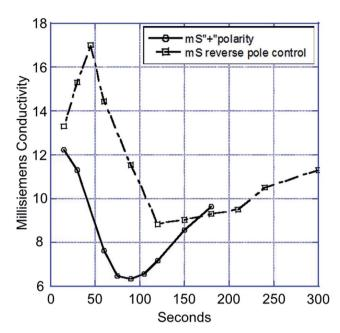
Fig. 31 Electrosorption process for the capacitor based on an ionic group derivatized nanoporous carbon electrode charged in the positive polarity and scientific control capacitor (Reproduced with permission from ref. 132.)
