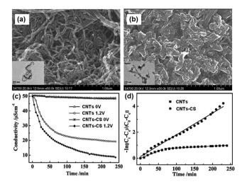
**Fig. 23** SEM images of (a) CNTs and (b) CNTs–CS. The insets are their TEM images. (c) Variation of solution conductivity with time and (d) linear plot of the pseudo-first-order kinetic equation for the electrosorption of Cu<sup>2+</sup> by CNTs and CNTs–CS. (Reproduced with permission from ref. 59.)
