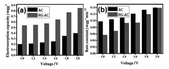
Fig. 8 (a) Electrosorption capacity of the AC and RG–AC (20 wt% RG) electrodes at different voltages in NaCl solution with an initial conductivity of 50  $\mu$ S cm<sup>-1</sup>; (b) rate constants of the electrosorption kinetics for AC and RG–AC (20 wt% RG) electrodes at different voltages. (Reproduced with permission from ref. 90.)
