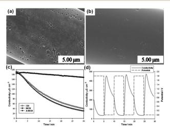
Fig. 29 SEM images of (a) the bare carbon cloth surface and (b) the embedded carbon electrode surface; (c) variations in the ion conductivity of the CDI, MCDI and A-MCDI during their operation; (d) continuous mode operation of the A-MCDI system by repeated adsorption and desorption cycles. (Reproduced with permission from ref. 147.)
