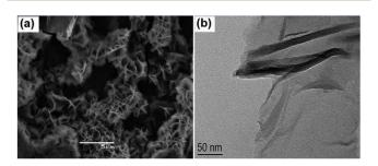
Fig. 6 (a) SEM and (b) TEM images of RG. (Reproduced with permission from ref. 46.)
