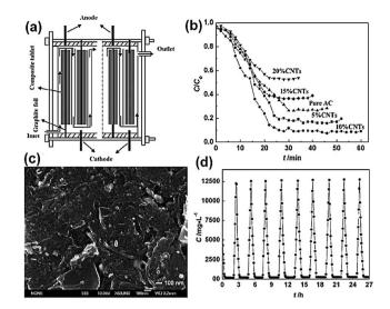
Fig. 3 (a) A schematic diagram of the flow-through capacitor apparatus; (b) comparison of the removal characteristics of the CNTs-AC composite electrodes; (c) SEM image of the composite electrode with 10 wt% CNTs; (d) removal and regeneration curve for the composite electrode with 10 wt% CNTs. (Reproduced with permission from ref. 65.)
