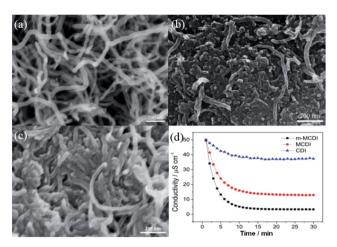
Fig. 30 SEM images of the (a) CNTs, (b) CNTs-PEI and (c) CNTs-DMDAAC electrodes; (d) electrosorption process for the CDI, MCDI, m-MCDI cells. (Reproduced with permission from ref. 144.)
