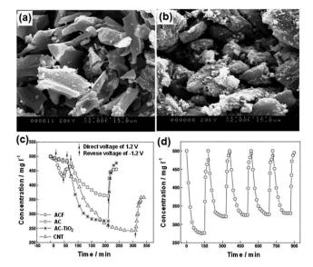
Fig. 15 SEM images of (a) AC and (b)  $AC-TiO_2$ ; (c) desalination and desorption curves for the different electrodes; (d) electrosorption and desorption cycles for the  $AC-TiO_2$  electrode. (Reproduced with permission from ref. 107.)
