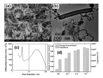
Fig. 5 (a) SEM and (b) TEM images of the CNTs-CNFs composite. (Reproduced with permission from ref. 75.) (c) Pore size distribution of the CNTs-CNFs composite. (Reproduced with permission from ref. 70.) (d) Electrosorption capacity and double layer capacitance of the CNTs-CNFs composite electrodes in different cation solutions. (Reproduced with permission from ref. 71.)
