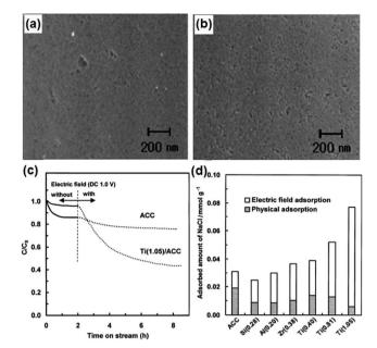
Fig. 14 SEM images of (a) ACC and (b) Ti (0.81)/ACC; (c) adsorption profiles of NaCl on the ACC and Ti (1.05)/ACC electrodes; (d) physical adsorption and electric field adsorption of the modified ACC electrodes. (Reproduced with permission from ref. 110.)
