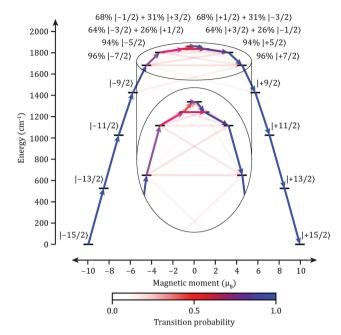
Fig. 3 Electronic states and magnetic transition probabilities for the ground  ${}^{6}H_{15/2}$  multiplet of **2** in zero field. The x-axis shows the magnetic moment of each state along the main magnetic axis of the molecule. Relaxation commences from the  $|-15/2\rangle$  state and only includes pathways which reverse the magnetization. Relaxation probabilities are calculated based on a magnetic perturbation and are normalized from each departing state (see ESI† for details).
