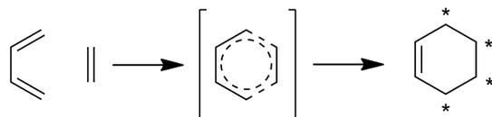
Fig. 13 The Diels–Alder reaction. [4 + 2]-cycloaddition between a diene and a dienophile proceeds through a pericyclic six-membered ring transition state to form a cyclohexene product. Asterisks indicate the stereocenters in the product which can be generated through Diels–Alder cycloaddition if the substrates bear the appropriate substituents.
