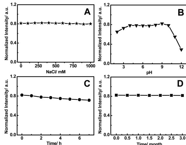
**Fig. 4** (A) The relative fluorescence intensity at  $427\text{ nm}$  (excitation at  $344\text{ nm}$ ) of the FNCPs in the  $\text{NaCl}$  solution. (B) Dependence of the fluorescence intensity on the pH values from  $2$  to  $12$ . (C) The variation of the fluorescence intensity of the FNCPs under irradiation by a  $500\text{ W}$   $\text{Xe}$  lamp for different time intervals. (D) Photostability of the FNCPs as a function of the storage time.
