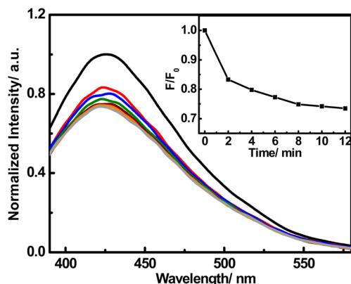
**Fig. 5** Time-dependent fluorescence responses of the FNCPs to 50  $\mu\text{M}$   $\text{Hg}^{2+}$ . Inset shows the  $F/F_0$  plotted against time in the presence of 50  $\mu\text{M}$   $\text{Hg}^{2+}$ , where  $F$  and  $F_0$  are the fluorescence intensity of the FNCPs at 427 nm with and without  $\text{Hg}^{2+}$ , respectively.
