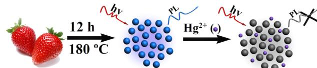
**Scheme 1** Schematic illustration of the preparation process for the FNCPs and their application for  $Hg^{2+}$  detection.
