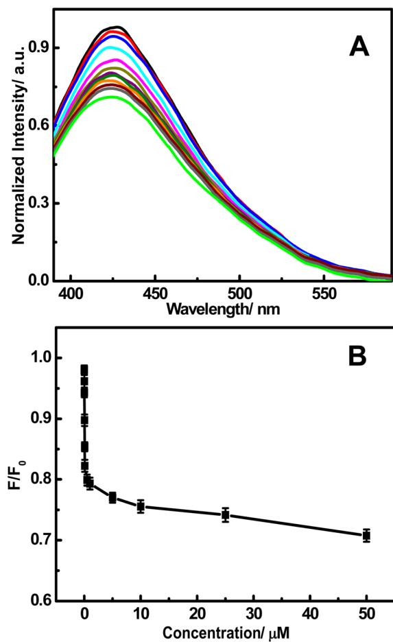
**Fig. 7** (A) The fluorescence responses of the FNCPs in a phosphate solution (25 mM, pH 7.4) after the addition of different concentrations of  $\text{Hg}^{2+}$  (top to bottom): 0, 0.010, 0.025, 0.050, 0.075, 0.100, 0.500, 1.00, 5.00, 10.0, 25.0, and 50.0  $\mu\text{M}$ . (B) Plot of the  $F/F_0$  with the concentration of  $\text{Hg}^{2+}$ .
