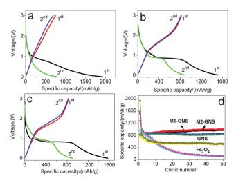
**Fig. 9** The initial two charge/discharge curves of (a) original GNS, (b) M1-GNS and (c) M2-GNS, and (d) cycling performance of M1-GNS, M2-GNS, GNS, and Fe<sub>3</sub>O<sub>4</sub> nanoparticles at the current density of 50 mAg<sup>-1</sup>.
