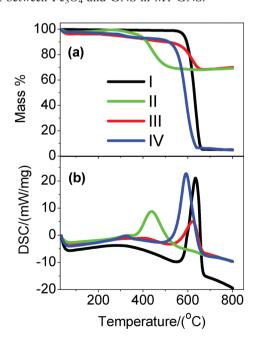
Fig. 5 (a) TG and (b) DSC curves of (I) GNS, (II) M1-GNS, (III) M2-GNS, and (IV) graphene sheets obtained from M1-GNS after removing the Fe<sub>3</sub>O<sub>4</sub> using HCl (1 mol/L).
