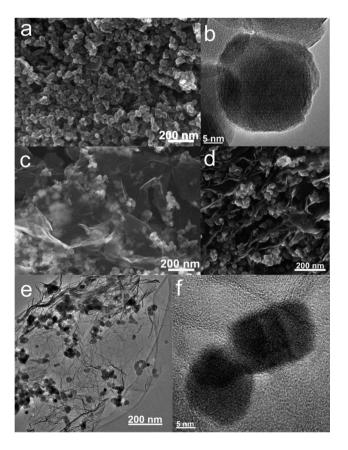
Fig. 4 (a) SEM and (b) HRTEM images of commercial Fe<sub>3</sub>O<sub>4</sub> nanoparticles; and (c, d) SEM, (e) TEM, and (f) HRTEM images of M2-GNS.
