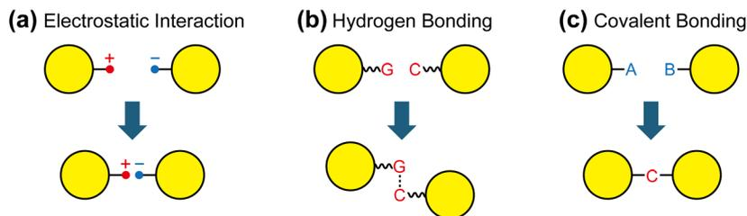
Fig. 1 Assembly of AuNPs through molecular interactions: (a) electrostatic attraction between oppositely charged surface groups (e.g.,  $-\text{NH}_3^+/-\text{COO}^-$ ), (b) hydrogen bonding between complementary functional groups (e.g., DNA bases), and (c) covalent bond formation through chemical reactions between surface ligands.
