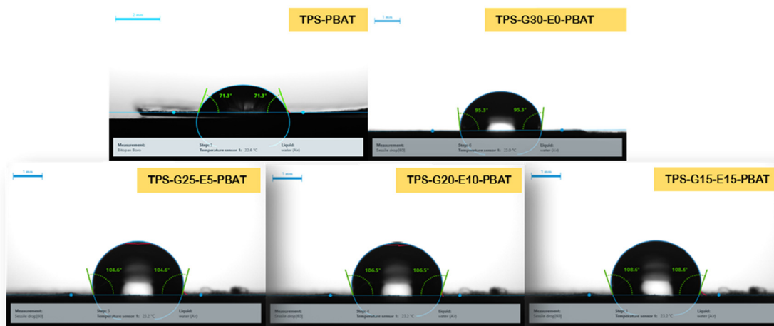
Fig. 4 Contact angle of the composite thin films.
