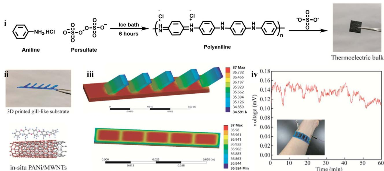
**Fig. 21** (i) Synthesis route of the thermoelectric generator. (ii and iii) Image and simulated thermal profile of thermoelectric generators, with (iv) showing the voltage output when the device was applied to the forearm. Reproduced with permission from ref. 278. Copyright 2021, Royal Society of Chemistry.
