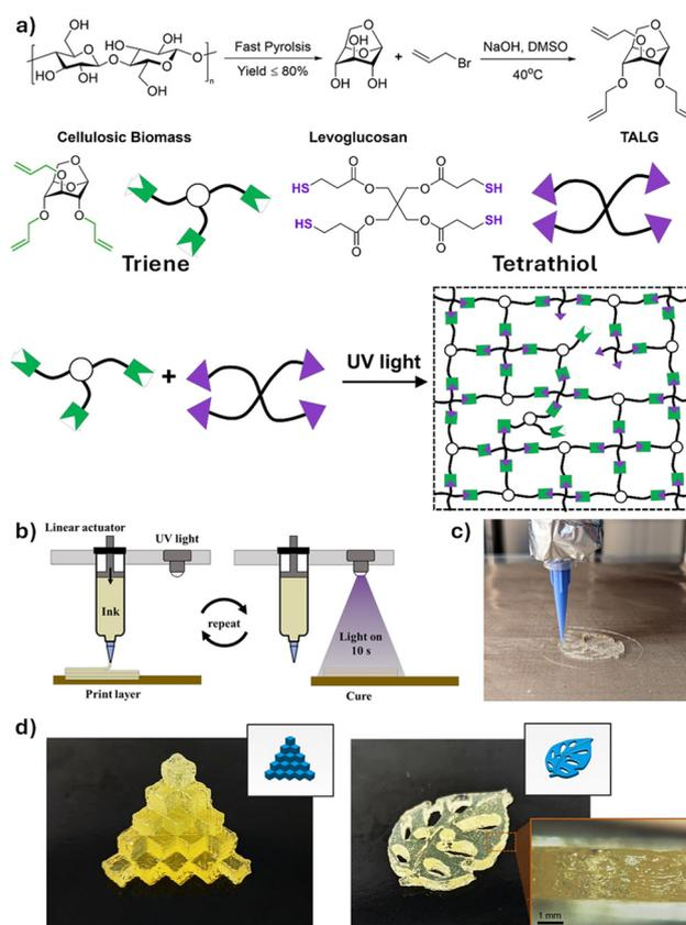
**Fig. 14** (a) Schematic diagram of DIW 3D printing ink with triene and tetrathiol as the main components and its photopolymerization reaction. (b) A schematic illustration of the DIW process used for 3D printing. (c) Real-time image capturing the extrusion of TALG-poly3SH-1 resin during printing. (d) Representative 3D printed structures fabricated using the TALG-poly3SH-1 formulation. Reproduced with permission from ref. 181. Copyright 2023, Royal Society of Chemistry.
