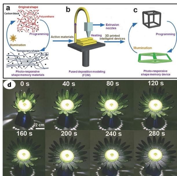
**Fig. 4** (a) Photoresponsive shape-memory behavior of carbon black–PU composite. (b) Fabrication of 3D-printed structures via FDM, where controlled layer-by-layer deposition occurs on a glass substrate. (c) Light-triggered shape recovery of the 3D-printed device. (d) Displaying the deformation of photosensitive printed sunflowers transitioning from bud to bloom under light exposure. Scale bar represents 2 centimeters. Reproduced with permission from ref. 69. Copyright 2017, Wiley.
