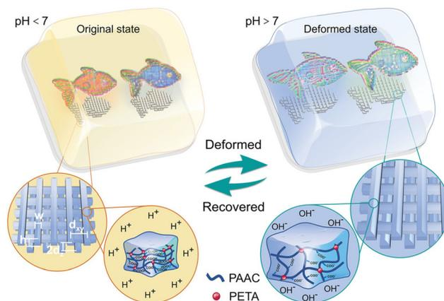
**Fig. 3** Schematic of pH-responsive color and shape changes in 4D printed woodpile microstructures. Vivid structural colors appear at pH < 7, while swelling at pH > 7 due to electrostatic repulsion between ionized carboxylate groups alters the lattice and fades the color. This transition is fully reversible upon pH restoration. Reproduced with permission from ref. 61. Copyright 2023, Wiley.
