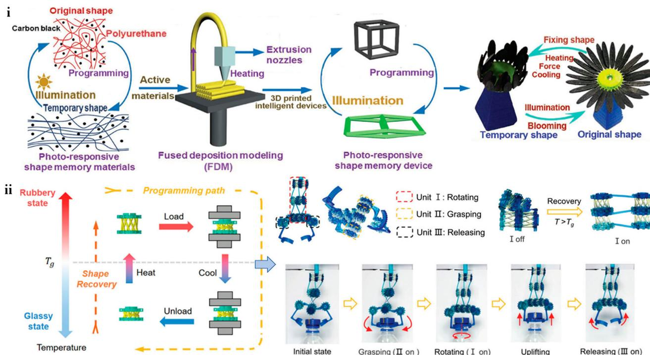
**Fig. 23** (i) FDM-printed SMP flower with carbon black, activated by visible light. Reproduced with permission from ref. 69. Copyright 2017, Wiley-VCH. (ii) 3D-printed SMP pressure-twist units assembled into a versatile soft gripper. Reproduced with permission from ref. 322. Copyright 2023, Wiley-VCH.
