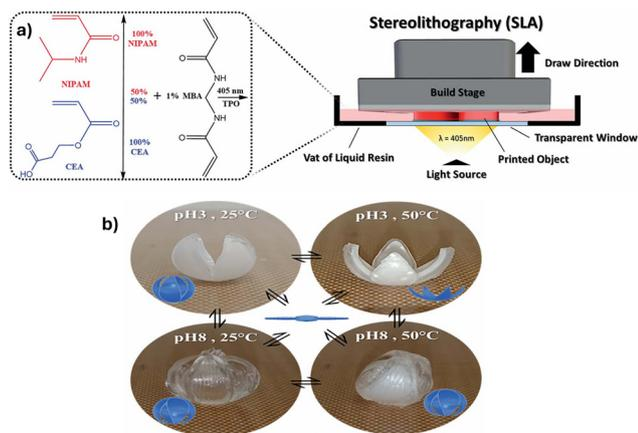
**Fig. 7** (a) Schematic representation of the chemical components and rapid bottom-up fabrication of gradient-like structures through photopolymerization of NIPAM and CEA using TPO as the photoinitiator and MBA as the crosslinker. (b) Demonstration of dual-responsive actuation to temperature and pH in 3D-printed gradient-like hydrogels with compositionally varied layers across the structure. Reproduced with permission from ref. 84. Copyright 2019, Royal Society of Chemistry.
