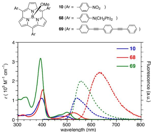
Fig. 5 UV-vis absorption (solid line) and fluorescence (dashed line) spectra of subporphyrins **10**, **68**, and **69** bearing 4-substituted phenyl groups at the *meso*-positions in  $\text{CH}_2\text{Cl}_2$ .
