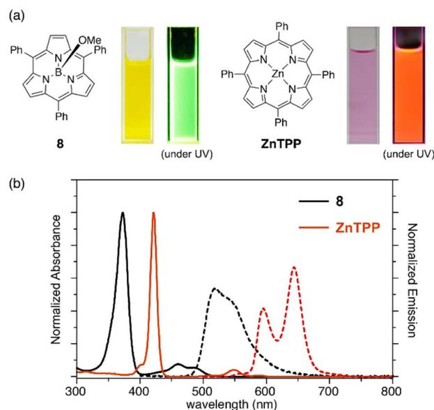
Fig. 4 (a) Photographs of  $\text{CH}_2\text{Cl}_2$  solutions of **8** and ZnTPP under room light and UV light. (b) UV-vis absorption (solid line) and emission (dashed line) spectra of subporphyrin **8** and tetraphenylporphyrin (ZnTPP) in  $\text{CH}_2\text{Cl}_2$ .
