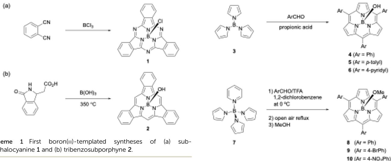
Scheme 1 First boron(III)-templated syntheses of (a) subphthalocyanine **1** and (b) tribenzosubporphyrine **2**.
