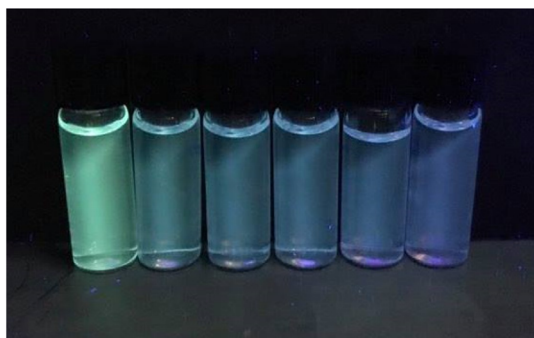
Fig. 6 Solutions of receptor 6 with increasing amounts of caffeine 30 under irradiation with UV light. \lambda_{\text{ex}} = 365 \text{ nm} ; [\mathbf{6}] = 5 \mu\text{M} ; solvent = 10 mM aqueous phosphate buffer, [\mathbf{30}] (left to right) = 0 mM, 2.5 mM, 5 mM, 10 mM, 20 mM, 40 mM.
