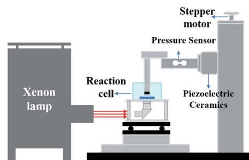
Fig. 6 Schematic diagram of the photoelectric-effect-accelerated ECNL instrument.
