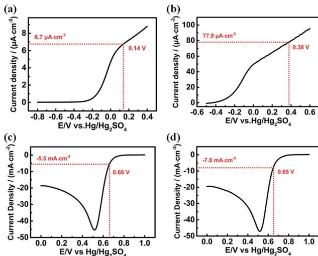
Fig. 2 Linear scan voltammograms of the n-GaAs electrode and Pt electrode at a scan rate of 100 mV s<sup>-1</sup>: (a) and (c) in the dark; (b) and (d) under illumination. The aqueous solution contains 40 mM KMnO<sub>4</sub> and 1.84 M H<sub>2</sub>SO<sub>4</sub>. The working temperature is kept at 25 °C and the illumination power is 460 mW.
