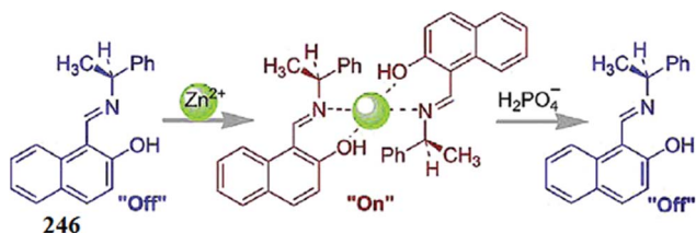
Fig. 210 Chemical structure of receptor 246, proposed ligand–zinc complexation mechanism and reversibility.
