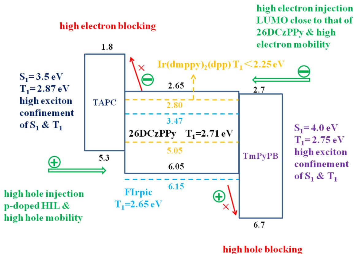
**Figure 3.** The charge/exciton confining structure for device W1 and the schematic diagram of EL procedures.
