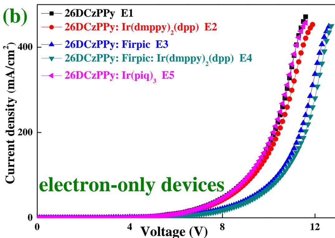
**Figure 5.** The J-V characteristics of single-charge transport devices with guests FIrpic, Ir(dmppy)<sub>2</sub>(dpp), (MPPZ)<sub>2</sub>Ir(acac) and Ir(piq)<sub>3</sub>-doped the host 26DCzPPy. a) hole-only devices. b) electron-only devices.
