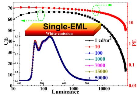
The simplicity/ extremely high efficiency/ low efficiency roll-off/ stable color trade-off has been accomplished in a single-EML WOLED.
