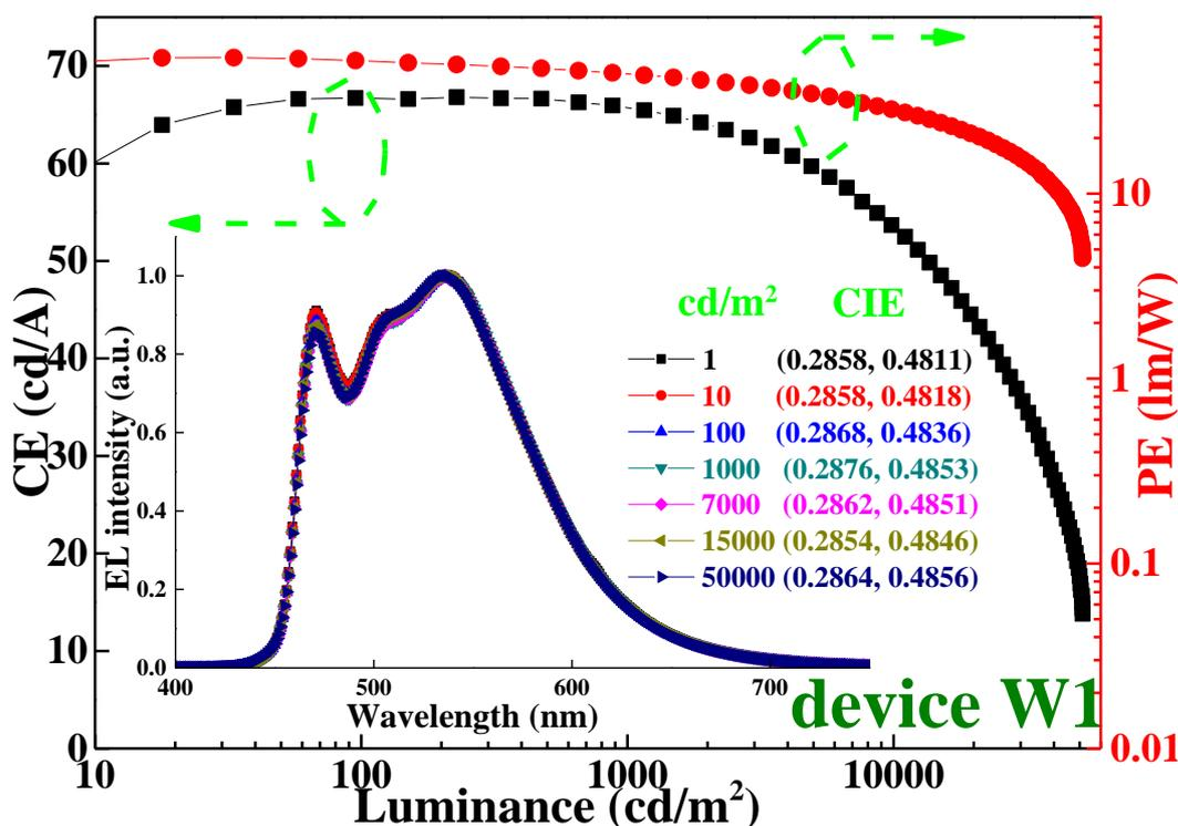
**Figure 2.** Forward-viewing CE and PE in dependence of luminance for device W1.
