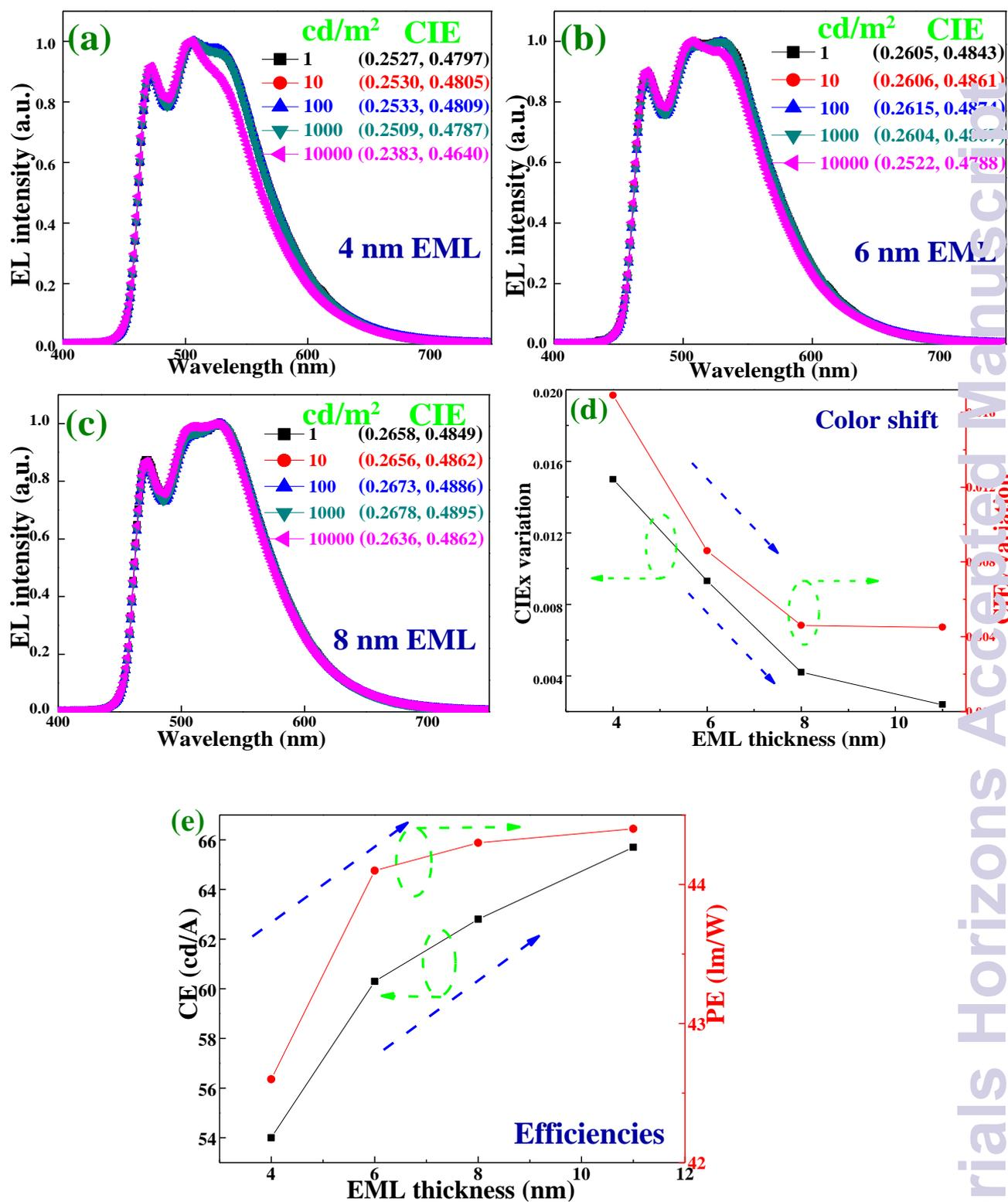
**Figure 4.** Normalized EL spectra of the devices comprising various EML thicknesses during 1- 10000  $\text{cd m}^{-2}$ : a) 4 nm. b) 6 nm. c) 8 nm. d) The color variation as a function of EML thickness. e) Forward-viewing efficiencies at 1000  $\text{cd m}^{-2}$  as a function of EML thickness.
