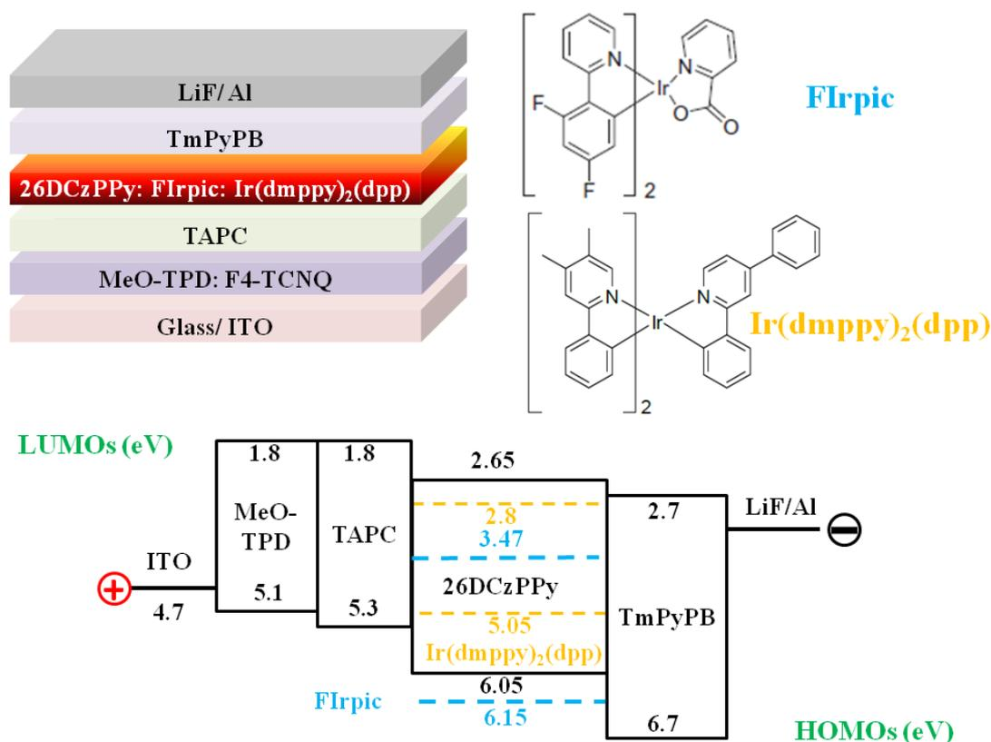
**Figure 1.** Top: The structure of W1 and the chemical structure of guests. Bottom: The proposed highest occupied molecular orbital (HOMO) and lowest unoccupied molecular orbital (LUMO) of the device.
