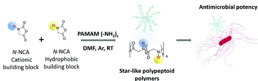
Fig. 24 Design and synthesis of antibacterial star-like \alpha -peptoid polymers. Reproduced from ref. 88 with permission from the Royal Society of Chemistry.
