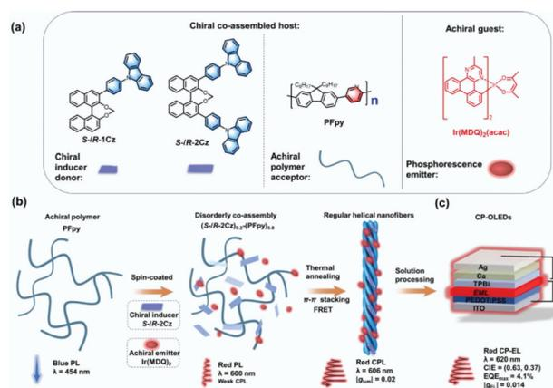
Fig. 11 (a) Chemical structures of *S/R*-1Cz, *S/R*-2Cz, PFpy, and Ir(MDQ)<sub>2</sub>. (b) Schematic diagram of the route to a red CPL. (c) The device structure of the CP-OLEDs. Reproduced with permission.<sup>60</sup> Copyright 2023, Wiley-VCH.
