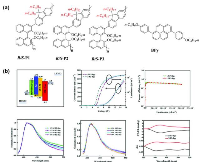
**Fig. 12** (a) Chemical structures of *R/S*-P1, *R/S*-P2, *R/S*-P3 and BPy. (b) The device structure of the CP-PLEDs, and *J*-*V*-*L*, CE, EL spectra of the *R*-P2-Bpy device, EL spectra of the *S*-P2-Bpy device and the CPEL curves. Reproduced with permission.<sup>61</sup> Copyright 2021, Royal Society of Chemistry.
