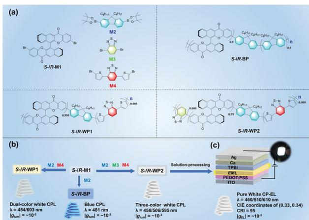
**Fig. 4** (a) Chemical Structures of S-/R-M1, S-/R-BP, S-/R-WP1, and S-/R-WP2; (b) Schematic diagram of the route for blue and white CPL; (c) Device configuration of the CP-PLEDs. Reproduced with permission.<sup>35</sup> Copyright 2022, Wiley-VCH.
