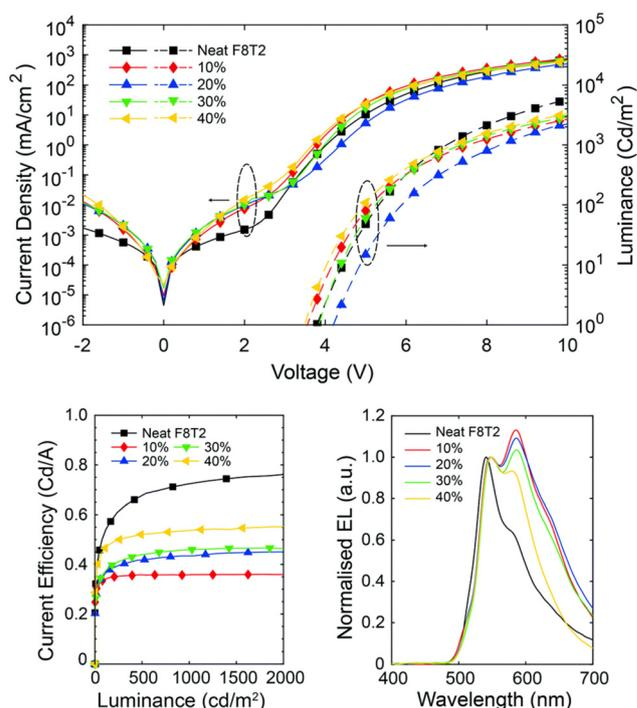
Fig. 8  $J$ - $V$ - $L$ , CE and PE spectra of F8T2:aza[6]H devices with increasing active layer thickness. Reproduced with permission.<sup>53</sup> Copyright 2022, Royal Society of Chemistry.
