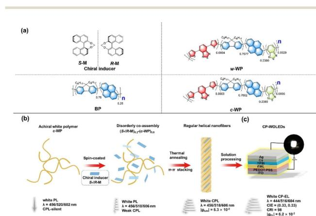
Fig. 10 (a) Chemical structures of *S/R*-M, BP, w-WP and c-WP. (b) Schematic diagram of the route to a white CPL. (c) Device structure of the CP-WOLEDs. Reproduced with permission.<sup>59</sup> Copyright 2023, Wiley-VCH.
