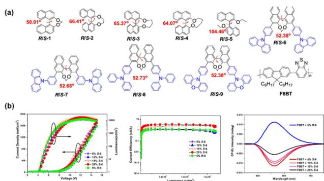
Fig. 9 (a) Chemical structures of *R/S*-1–*R/S*-9 and F8BT. (b)  $J$ - $V$ - $L$ , CE and CPEL spectra of devices based on blends of F8BT with various amounts of *R/S*-6. Reproduced with permission.<sup>54</sup> Copyright 2021, American Chemical Society.
