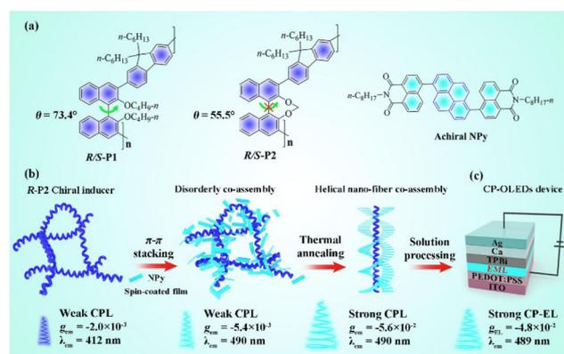
**Fig. 13** (a) Chemical structures of *R/S*-P1, *R/S*-P2 and NPy. (b) Schematic diagram of the possible co-assembly route for (*R*-P2)<sub>0.6</sub>(NPY)<sub>0.4</sub>. (c) Device structure of the CP-PLEDs. Reproduced with permission.<sup>63</sup> Copyright 2022, Wiley-VCH.
