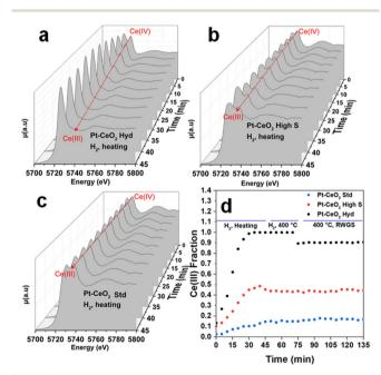
Fig. 4 Time evolution of the in situ XANES spectra at the Ce L<sub>3</sub> edge during heating treatment to 400  $^{\circ}\text{C}$  under  $\text{H}_2$  atmosphere for a) Pt-CeO<sub>2</sub> Hyd, b) Pt-CeO<sub>2</sub> high S and c) Pt-CeO<sub>2</sub> Std samples. d) Time evolution of the Ce(III) fraction in the Pt-CeO2 samples during reduction and RWGS reaction.
