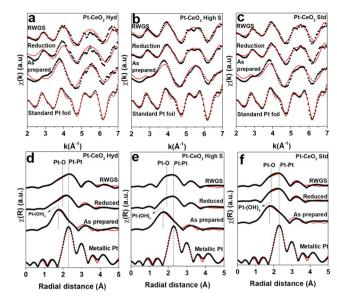
Fig. 5 EXAFS oscillations from *in situ* EXAFS measurements at the Pt  $L_3$  edge of the as-prepared Pt-CeO<sub>2</sub> samples, during reduction treatment and RWGS reaction (a-c) and the respective Fourier transform (d-f). The best fitting found is represented by the red line.
