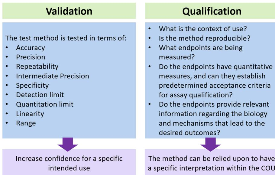
**Fig. 3** Illustration depicting the difference between qualification and validation. Both approaches are utilized to assess the capacity of MPS in ensuring the safety and effectiveness of biological products within the given context.
