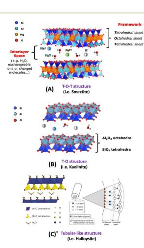
Fig. 1 Schematic view of different clay structures: T-O-T (A), T-O (B) structures and tubular-like structure (C\* is adapted with permission from ref. 1, Copyright 2020 MDPI).
