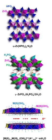
Fig. 2 Schematic view of  $\alpha$ -ZrP,  $\gamma$ -ZrP and LDHs structures.
