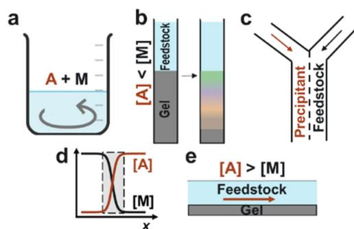
**Fig. 1** Schematics of precipitation-based separation methods. (a) Bulk mixing of the precipitating agent (A) and feedstock (M) solutions, (b) precipitation chromatography and (c) laminar co-flow separations, (d) steep concentration gradients at liquid–liquid interface, (e) proposed flow-gel method for rapid separations.
