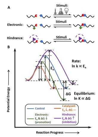
Fig. 2 (A) Generic dynamic covalent chemistry scheme related to equilibrium control through electronic/steric effects. (B) Control of reaction equilibrium and rate (rate constant: *k*) *via* steric hindrance and electronic effects. Blue: control. Orange: catalyzed. Green: electronic effects (promote the reaction in this case). Purple: steric effects (inhibit the reaction in the case shown in (A)).
