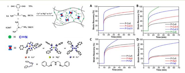
Fig. 6 (Left) Polyimine-metal complex vitrimers synthesized from terephthaldehyde (TPA), diethylenetriamine (DETA), and tris(2-aminoethyl) amine (TREN). (Right) Strain recovery curves to show the creep response of the polyimine-metal complex vitrimers at (A) 60 °C, (B) 80 °C, (C) 100 °C, and (D) 120 °C. Adapted from ref. 127 with permission from the American Chemical Society, copyright 2020.
