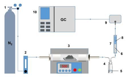
Fig. 1 The self-designed equipment for the thermochemical experiment (1. Nitrogen cylinder, 2. Gas flowmeter, 3. Glass tube furnace, 4. Gaswashing system, 5. Saturated sodium bicarbonate, 6. Skimmed cotton, 7. Drying tube, 8. Discolored silica gel, 9. Gas sample collection bag, 10. Gas chromatograph instrument).
