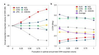
**Fig. 6** Performance of imported and exported volume (a) and LCOH (b) in RCEP members under the fluctuations in the optimal value of the annual total OWH exported volume. In (a), positive numbers represent exports and negative numbers represent imports.
