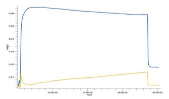
Fig. 6 Trend analysis of furfural reduction for the scale-up reduction. Wavenumbers selected:  $1713 \text{ cm}^{-1}$  (blue) to acetone and  $1680 \text{ cm}^{-1}$  (yellow) for the aldehyde. Reaction conditions: a 0.25 M solution of furfural in iso-propanol was pumped through a BZC column at  $120 \,^{\circ}\text{C}$  and 50 s residence time for 5.5 hours.
