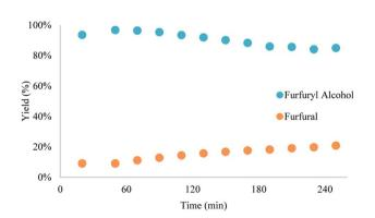
Fig. 5 Results of the scale-up reduction of furfural, with slight decrease in catalytic activity. Reaction conditions: a  $0.25 \,\mathrm{M}$  solution of furfural in iso-propanol was pumped through a BZC column at  $120 \,\mathrm{^{\circ}C}$  and  $50 \,\mathrm{s}$  residence time for  $5.5 \,\mathrm{hours}$ .
