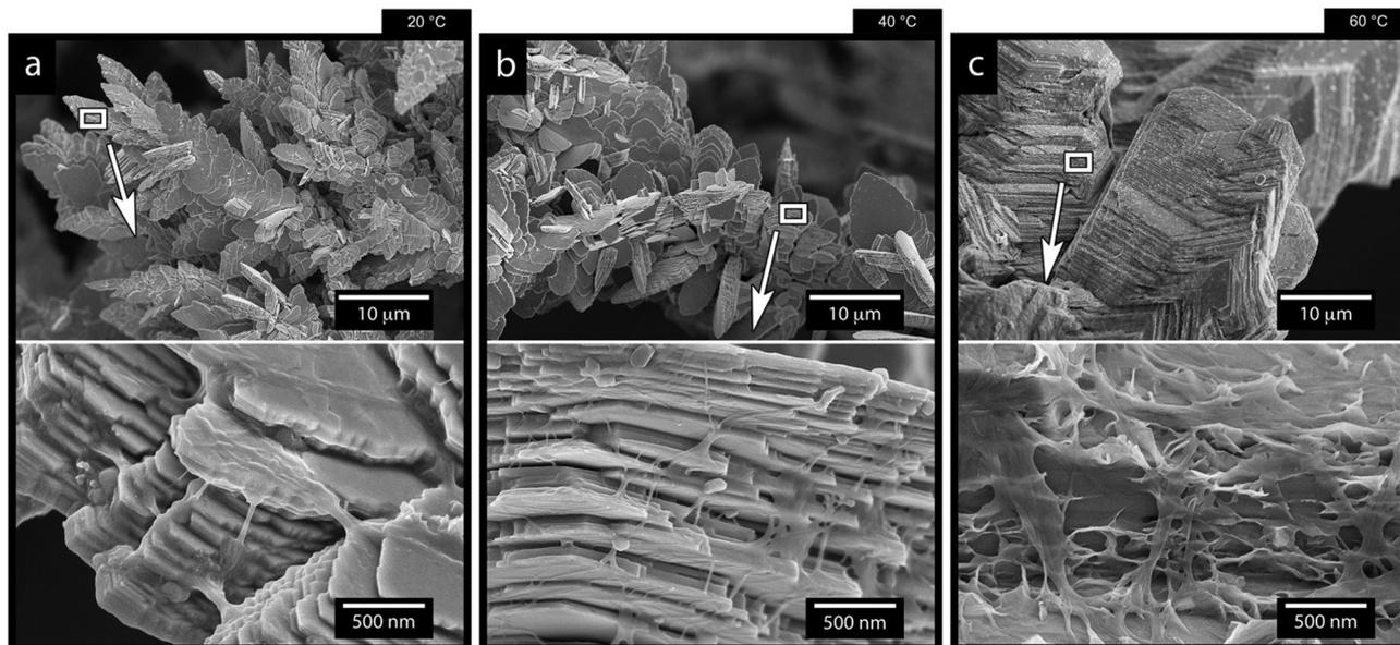
Fig. 9 SEM micrographs of the zinc electrodeposited Ti-electrodes after 7 min of electrodeposition at a current density of  $1000 \text{ A m}^{-2}$ , a CNF concentration of  $0.5 \text{ g L}^{-1}$ , and temperatures of  $20 \text{ }^\circ\text{C}$  (a),  $40 \text{ }^\circ\text{C}$  (b) and  $60 \text{ }^\circ\text{C}$  (c). A figure serving as the reference, describing the electrodeposition in the absence of cellulose at different temperatures are provided in Fig. S15 (ESI<sup>†</sup>).
