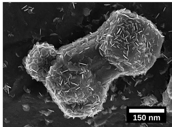
Fig. 4 Micrograph showing zinc electrodeposited after 5 s near one of the edges of the electrode using a current density of  $150 \text{ A m}^{-2}$ . The hexagonal nanoflakes are visible as merging with its surface.
