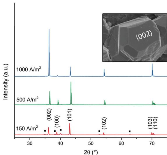
Fig. 3 XRD diffractograms of zinc deposited at current densities of  $150 \text{ A m}^{-2}$ ,  $500 \text{ A m}^{-2}$  and  $1000 \text{ A m}^{-2}$ . The peaks corresponding to the titanium phase (JCPDS-ICDD, 44-1294) are labelled with a black square (■). The hexagonal prism analogous to the zinc crystal in Fig. 1f illustrates the corresponding directions of the crystal planes (002) and (100).
