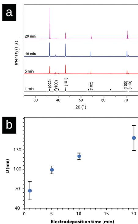
Fig. 5 (a) XRD patterns of zinc-deposition on the surface of the Ti substrate at a current density of  $1000 \text{ A m}^{-2}$  depending on electrodeposition times. 1 min (black); 6 min (red); 10 min (blue); and 20 min (pink). The peaks corresponding to titanium are labeled with a black square (■). (b) Crystallite size (*D*) as estimated with the Scherrer equation measured for four different electrodeposition times at a current density of  $1000 \text{ A m}^{-2}$ .
