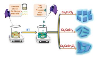
Fig. 1 Schematic illustration of the water-assisted synthesis of blue fluorescent Cs<sub>2</sub>CuCl<sub>4</sub> square nanoplates, Cs<sub>2</sub>CuBr<sub>4</sub> nanorods, and Cs2CuBr2Cl2 rectangular nanoplates
