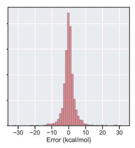
Fig. 8 Histogram of the errors in our fast estimator of zpe-corrected reaction barrier height  $\Delta E_{\rm o}$  relative to high-accuracy CCSD(T)-F12a/cc-pVDZ-F12//wB97X-D3/def2-TZVP values for about 2000 reactions not included in the training set. The mean absolute error in the estimates is <3 kcal mol<sup>-1</sup>, smaller than the average error in DFT calculations of these barriers.
