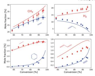
Fig. 13 Predictions of a large kinetic model for the outlet composition from steam cracking of propane vs. experimental measurements, after replacing 12 important rate coefficients in the model with high accuracy k(T,P). Reproduced from Faraday Discussions (https://doi.org/10.1039/d2fd00032f) with permission from the Royal Society of Chemistry.
