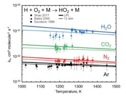
Fig. 1 Predicted vs. experimental rate coefficients for  $H + O_2 + M \rightarrow HO_2 + M$  near the low-pressure limit, showing how well Jasper's *ab initio* method works for predicting the dependence on bath gas composition (the identity of M). Reproduced from *Faraday Discussions* (https://doi.org/10.1039/d2fd00038e) with permission from the Royal Society of Chemistry.
