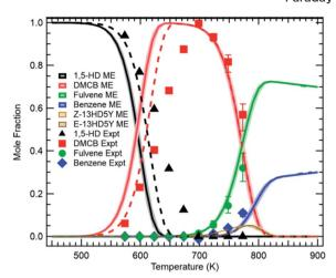
Fig. 9 Direct measurements of  $C_6H_6$  isomers formed from 1,5-hexadiyne pyrolysis (points) versus model predictions after ref. 17 (curves). Reproduced from Faraday Discussions (https://doi.org/10.1039/d2fd00028h) with permission from the Royal Society of Chemistry.
