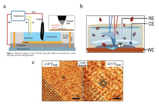
Fig. 5 (a) Schematic of *in situ* EC-STM setup. Copyright 2018, John Wiley and Sons; (b) schematic of *in situ* EC-AFM; (c) morphology of Cu surface at different potentials characterized by *in situ* AFM. Copyright 2020, John Wiley and Sons. All panels reproduced with permission. 139,143
