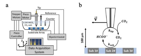
Fig. 4 (a) SECM operation principle; (b) the SG/TC mode all panels reproduced with permission.<sup>128</sup> Copyright 2020, Springer Nature.
