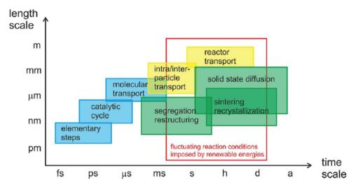
Fig. 3 Time scale of various processes in catalytic reactions. All panels reproduced with permission.<sup>29</sup> Copyright 2017, John Wiley and Sons.
