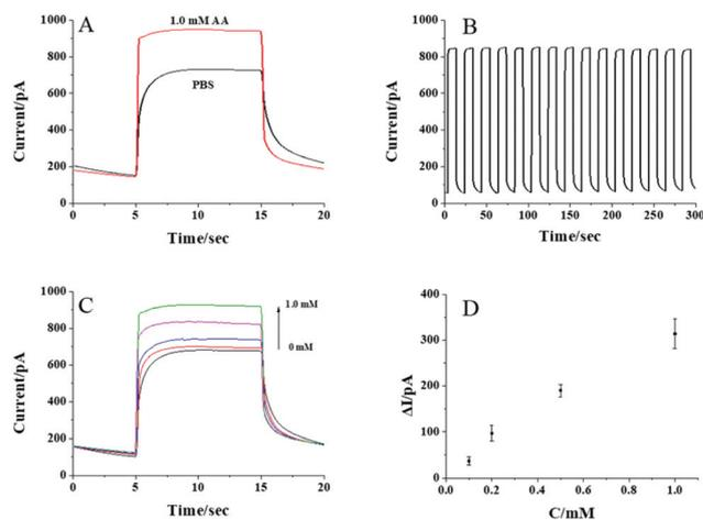
**Fig. 3** (A) Photocurrent traces of the CdS QD modified nanopipette in the presence and absence of 1 mM AA; (B) photocurrent stability of the CdS QD modified nanopipette in the presence of 1 mM AA; (C) photocurrent traces of AA at different concentrations (0, 0.1, 0.2, 0.5, 1 mM); (D) the linear response of the photocurrent to AA at different concentrations. The error bar presents the standard deviation from three CdS QD modified nanopipettes.
