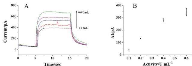
**Fig. 4** (A) Photocurrent traces of the CdS QD modified nanopipette in the presence of ALP with different activities (0, 0.1, 0.2, 0.4, 0.6 U mL<sup>-1</sup>); (B) the derived photocurrent response in the presence of ALP with different activities. The error bar presents the standard deviation from three independent measurements.
