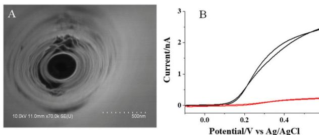
**Fig. 2** (A) The SEM image of the orifice of the nano-capillary after the sputtering of the ITO layer and coating with wax; (B) cyclic voltammograms of the nanopipette before (black curve) and after (red curve) modifying CdS QDs in 10 mM PBS with 5 mM  $K_4Fe(CN)_6$ . The scan rate is  $100\text{ mV s}^{-1}$ .
