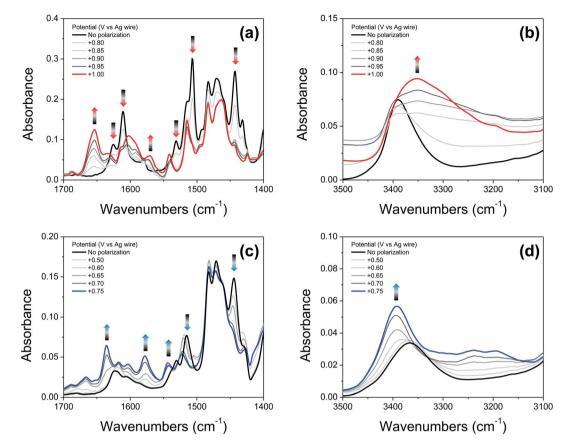
Fig. 6 (a and c): IRSEC spectra of 2' and 4', respectively, (19 mM solutions) polarized in 50 mV or 100 mV steps in the 1700–1400 cm<sup>-1</sup> region. (b and d): IRSEC spectra of 2' and 4', respectively, under the same conditions in the 3500–3100 cm<sup>-1</sup> region. Solvent: DCM, 0.1 M TBAPF<sub>6</sub>. Some of the characteristic bands showing changes upon electro-oxidation are indicated with upward and downward arrows.
