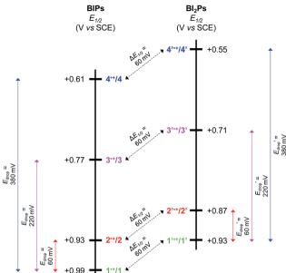
Fig. 5 Diagram showing the experimentally determined  $E_{1/2}$  for BIP derivatives (1–4) and BI<sub>2</sub>P analogs (1′–4′). The colored arrows show that the drop in  $E_{1/2}$  ( $E_{\rm drop}$ ) for the different TPAs is the same in both series. The dashed black arrows indicate the decrease in  $E_{1/2}$  ( $\Delta E_{1/2}$ ) due to the addition of one benzimidazole unit, which is 60 mV regardless of the TPA.
