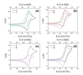
Fig. 4 (a–d) Cyclic voltammograms of Bl $_2$ Ps 1′–4′ (dashed lines). The cyclic voltammograms of analogous BIPs 1–4 (solid lines) are included for comparison. Concentration: 1 mM of the indicated compound, 0.5 M TBAPF $_6$  supporting electrolyte in dry acetonitrile. WE: glassy carbon. Pseudo RE: Ag wire (ferrocene as internal reference). CE: Pt wire. Scan rate, 100 mV s $^{-1}$ . Compound 3′ has low solubility in acetonitrile.
