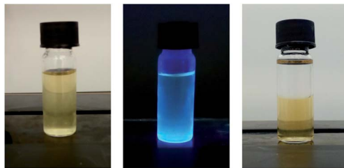
Fig. 8 Glucose-coated Si NPs in water under normal light (left) and 365 nm irradiation (middle). The right picture shows the solubility of glucose-coated Si NPs in hexane (top layer) and water (bottom layer).
