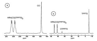
Fig. 1 <sup>13</sup>C NMR (a) and <sup>31</sup>P NMR (b) spectra of HRh(<sup>13</sup>CO)(TPPTS)<sub>3</sub> in the presence of a 3 molar excess of TPPTS under a 200 bar pressure of  $^{13}CO$ :  $H_2 = 1:1$  in  $D_2O$ . Modified with permission from ref. 59. Copyright of Springer (1989).
