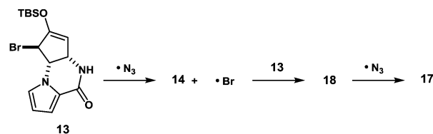
Scheme 3 Plausible mechanisms of the production of regioisomeric byproducts 17 and 18 .
