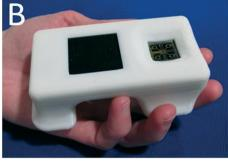
Fig. 1 (A) CAD design drawing of the handheld PCR. The illustration shows a display with a compartment accommodating 4 samples in the VRC form. (B) Fabricated and assembled complete real-time PCR device packaged within a 3D printed casing.
