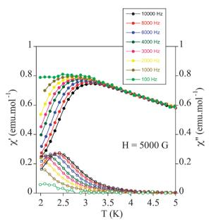
**Fig. 6** Temperature dependence of the in-phase AC susceptibility  $(\chi_m')$  (filled symbols) and the out-of-phase AC susceptibility  $(\chi_m'')$  (empty symbols) of **1** under an applied field of 0.5 T.
