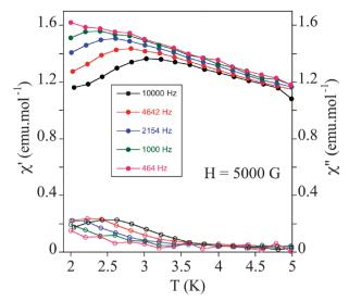
Fig. 8 Temperature dependence of the in-phase AC susceptibility  $(\gamma_m)'$ (filled symbols) and the out-of-phase AC susceptibility  $(\gamma_m)''$  (empty symbols) of 2 under an applied field of 0.5 T.
