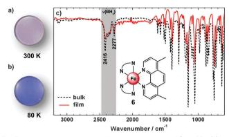
Fig. 5 Physical vapour deposited film on a quartz disc of 6 at 300 K (a) and 80 K (b), FT-IR spectra (c) of the bulk material (black dotted) and the vacuum deposited material (red) of 6 at 300 K
